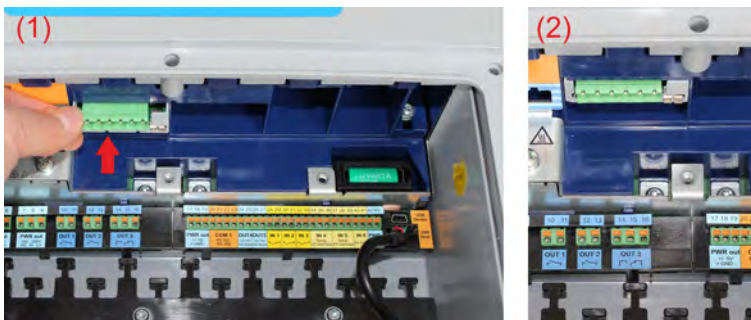
Fig. 96: Insert the option board
