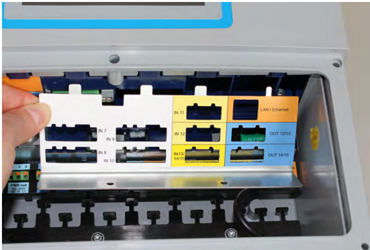
Fig. 95: Disassemble the cover plate
