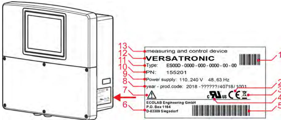
Fig. 3: Nameplate on device housing
