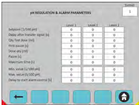
Fig. 62: Configuration -> Dosing Programm -> pH Regulation & alarms parameters
