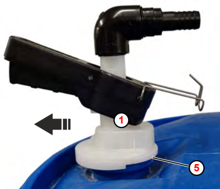
Fig. 13: Disconnect the connection coupling
