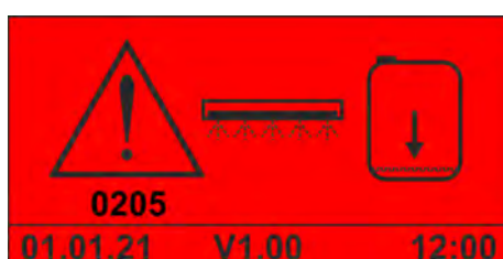
Fig. 25: Error code 205 (liquid rinse aid)
