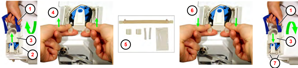
Fig. 21: Replacing the peristaltic hose
