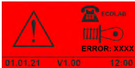
Fig. 31: Illustration 'measuring cell error'
